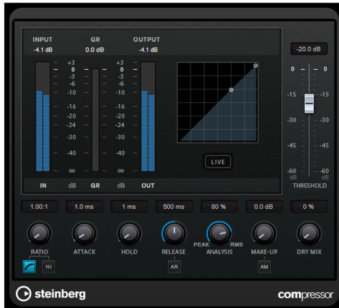
**Compressor** features a separate display that graphically illustrates the compressor curve that is shaped according to the **Threshold** and **Ratio** parameter settings. **Compressor** also features a
