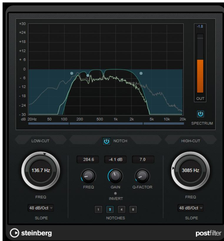
**PostFilter** combines a low-cut filter, a notch filter, and a high-cut filter. You can change the settings by dragging the curve points in the graphical display, or by adjusting the controls below the display section.
