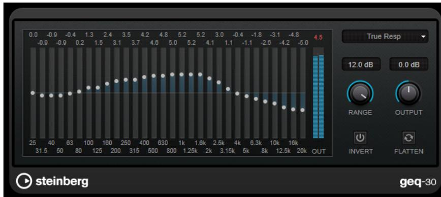
Each band can be attenuated or boosted by up to 12 dB, allowing for fine control of the frequency response. In addition, there are several preset modes available that can add color to the sound of **GEQ-10/GEQ-30**.
