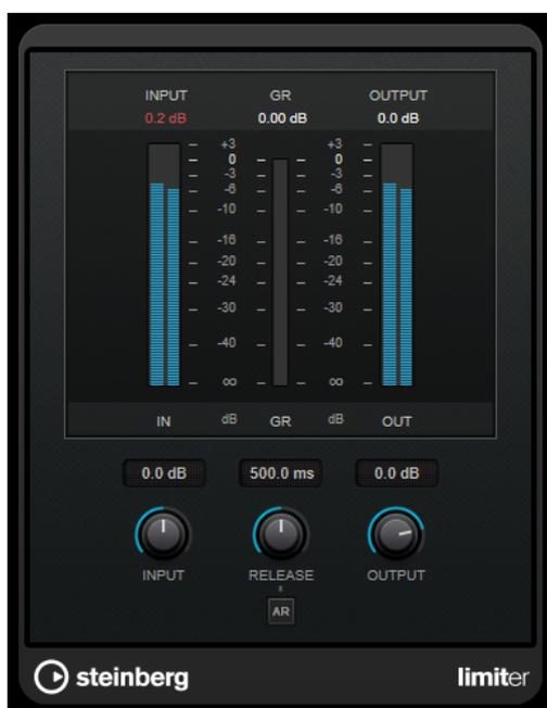
**Limiter** can adjust and optimize the **Release** parameter automatically according to the audio material, or it can be set manually. **Limiter** also features separate meters for the input, output and the amount of limiting (middle meters).
