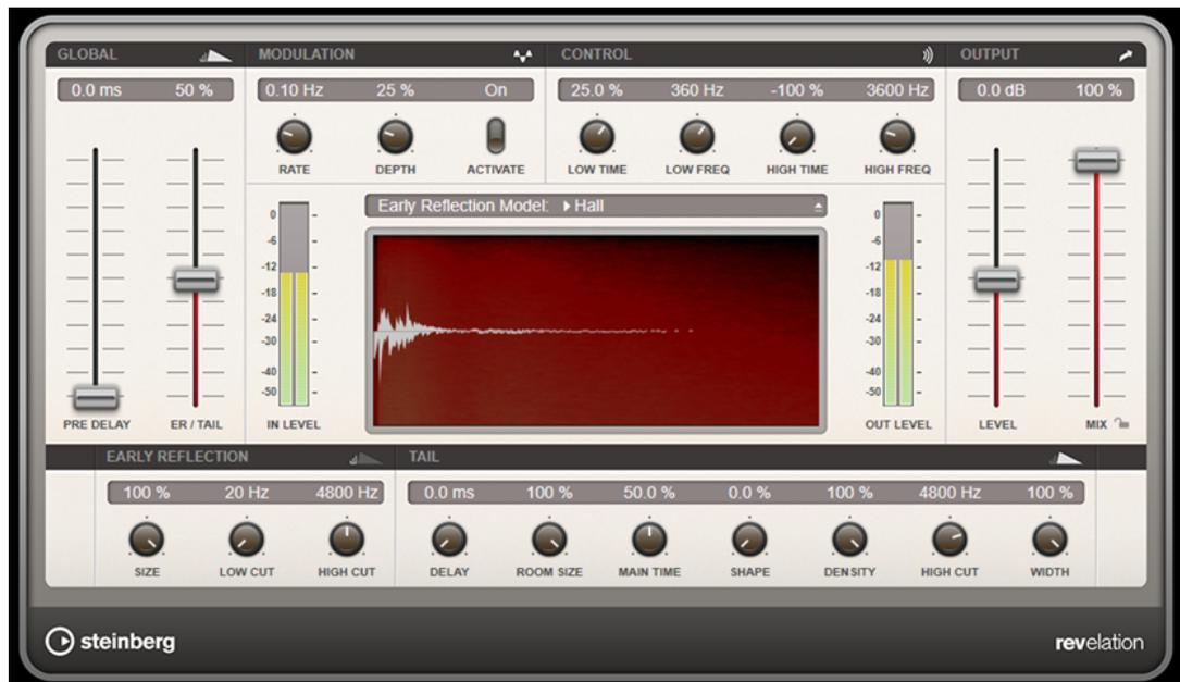
The early reflections are responsible for the spatial impression in the first milliseconds of the reverb. For emulating different rooms, you can choose between different early reflections patterns and adjust their size. The reverb tail, or late reverberation, offers parameters for controlling the room size and the reverb time. You can adjust the reverb time individually in 3 frequency bands.
