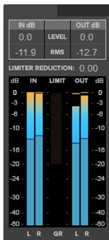
The input/output meter provides a combined peak level, with peak-hold functionality and RMS meter. Between the meters for input and output is the gain reduction meter for the **Limiter**.
