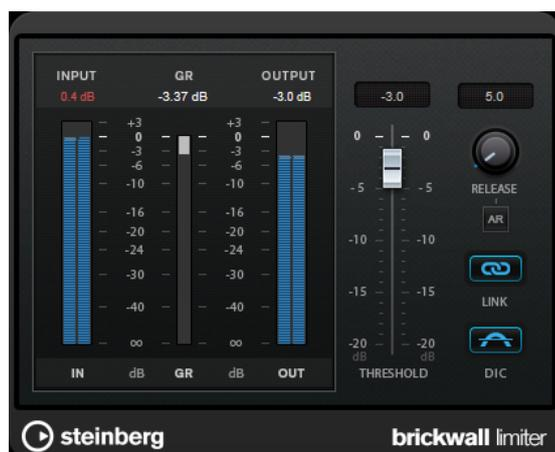
Due to its fast attack time, **Brickwall Limiter** can reduce even short audio level peaks without creating audible artifacts. However, this plug-in creates a latency of 1ms. **Brickwall Limiter** features separate meters for input, output, and the amount of limiting. Position this plug-in at the end of the signal chain, before dithering.
