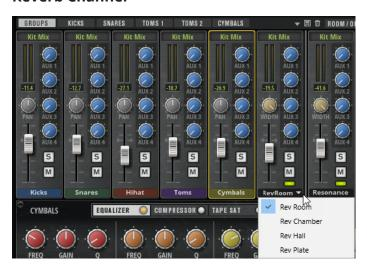
The **Reverb** channel on the **Groups** page provides the same controls as all other group channels. To select the reverb type, click on the channel name to open the **Select Reverb Type** pop-up menu, and select an option. You can choose from **Room**, **Chamber**, **Hall**, and **Plate**.
