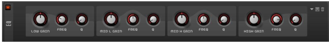
The two mid-range bands act as peak filters and the low and high bands act as shelving filters. All bands are fully parametric with adjustable **Gain**, **Frequency**, and **Q** parameters.
