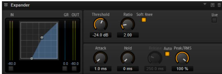
The graphical control to the left shows the expansion curve. You can edit the **Threshold** and **Ratio** values with the handles of this control. The input and output meters indicate the level before and after the expansion. The Gain Reduction meter indicates the current attenuation of the level.
