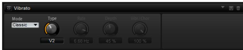
The effect provides direct access to the classic chorus and vibrato settings (C1, C2 and C3 and V1, V2 and V3). In addition, there is a custom mode that allows you to adjust the amount of chorus or vibrato freely.
