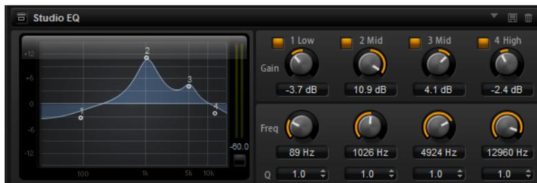
With the four frequency bands, you can shape the tone color, to create a brighter or darker sound, for example. The two mid-range bands act as peak filters and the low and high bands act as shelving filters. All bands are fully parametric with adjustable gain, frequency, and Q factor. Each frequency band offers the following controls:
