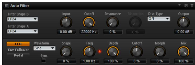
The morphing between the two shapes, as well as the cutoff, can be controlled with a manual pedal control, an LFO, or an envelope follower.
