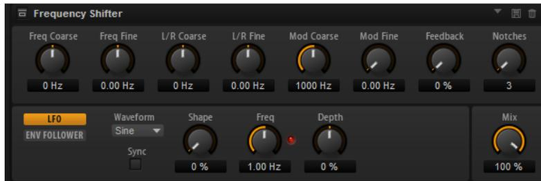
Unlike pitch shifters, where the frequencies are shifted by a factor, and where the harmonic relations are kept, a frequency shifter alters the harmonic relations. Therefore, a larger frequency shift usually results in a disharmonic sound.
