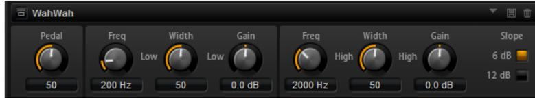
You can independently specify the frequency, width, and the gain for the low and high pedal positions. The crossover point between the low and high pedal positions lies at 50.
