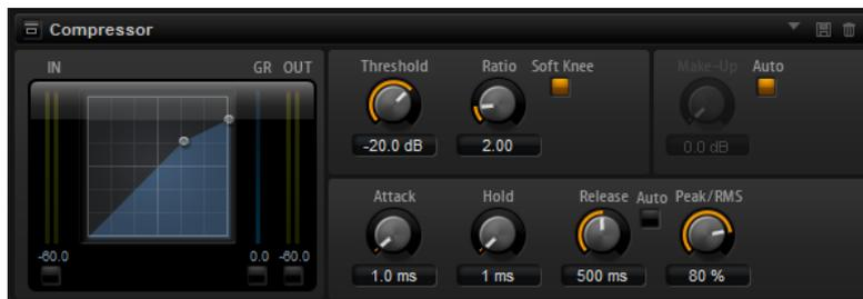
The graphical control to the left indicates the compression curve. You can edit the **Threshold** and **Ratio** values with the handles of this control. The input and output VU meters indicate the level before and after the compression. The Gain Reduction meter indicates the current attenuation of the level.
