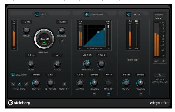
The window is divided into three sections containing controls and meters for each effect. Activate the individual effects using the **Gate**, **Compressor**, and **Limiter** buttons. You can select between three different routing options using the **Module Configurator** button.
