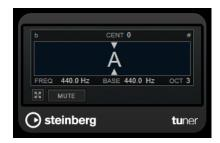
The graphical display indicates the currently played pitch as a note. The two arrows indicate any pitch deviation. The deviation is also shown in the upper area of the display. If the played note is flat of the pitch, the pitch indicator is located to the left. If the played note is sharp, the pitch indicator is located to the right.
