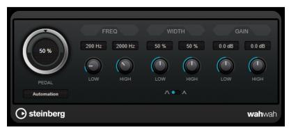
You can independently specify the frequency, width, and gain for the **Low** and **High** Pedal positions. The crossover point between the Lo and Hi Pedal positions lies at 50.
