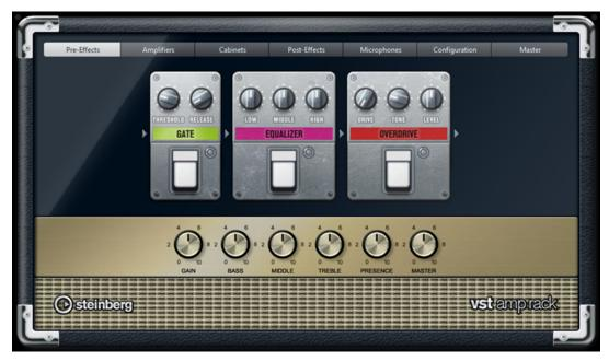
At the top of the plug-in panel, there are six buttons, arranged according to the position of the corresponding elements in the signal chain. These buttons open different pages in the display section of the plug-in panel: **Pre-Effects**, **Amplifiers**, **Cabinets**, **Post-Effects**, **Microphones**, **Configuration**, and **Master**.
