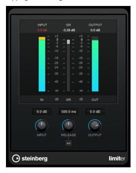
**Limiter** can adjust and optimize the **Release** parameter automatically according to the audio material, or it can be set manually. **Limiter** features separate meters for the input, output and the amount of limiting (middle meters).
