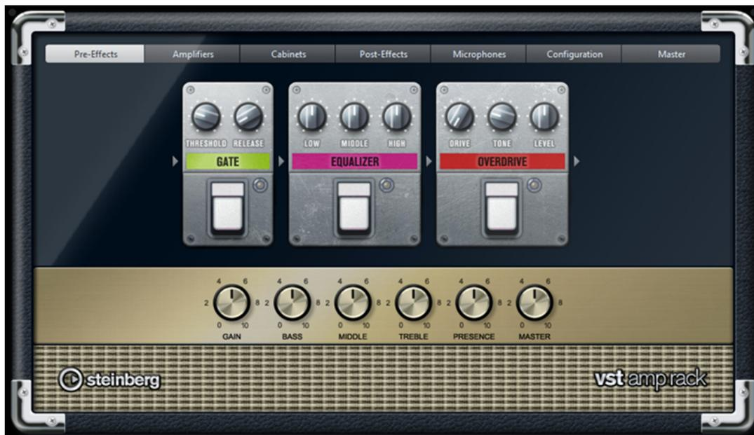
At the top of the plug-in panel, there are six buttons, arranged according to the position of the corresponding elements in the signal chain. These buttons open different pages in the display section of the plug-in panel: **Pre-Effects**, **Amplifiers**, **Cabinets**, **Post-Effects**, **Microphones**, **Configuration**, and **Master**.
