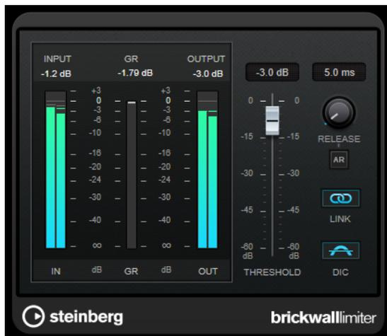
Due to its fast attack time, **Brickwall Limiter** can reduce even short audio level peaks without creating audible artifacts. However, this plug-in creates a latency of 1ms. **Brickwall Limiter** features separate meters for input, output, and the amount of limiting. Position this plug-in at the end of the signal chain, before dithering.
