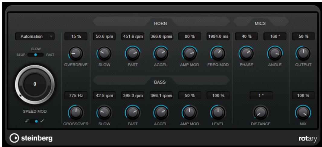
A rotary speaker cabinet features speakers rotating at variable speeds to produce a swirling chorus effect, commonly used with organs.
