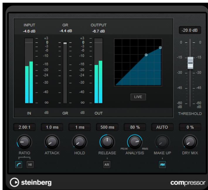
**Compressor** features a separate display that graphically illustrates the compressor curve that is shaped according to the **Threshold** and **Ratio** parameter settings. **Compressor** also features a **Gain Reduction** meter that shows the amount of gain reduction in dB, **Soft knee/Hard knee** compression modes, and a program-dependent auto feature for the **Release** parameter.
