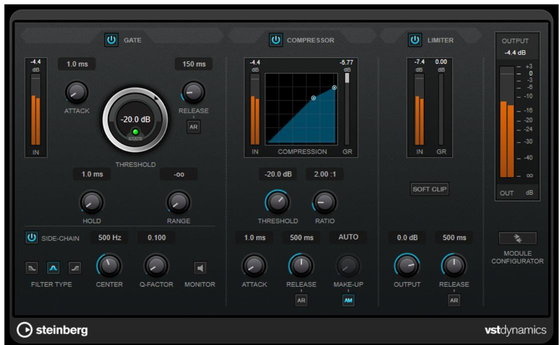
The window is divided into three sections containing controls and meters for each effect. Activate the individual effects using the **Gate**, **Compressor**, and **Limiter** buttons. You can select between three different routing options using the **Module Configurator** button.
