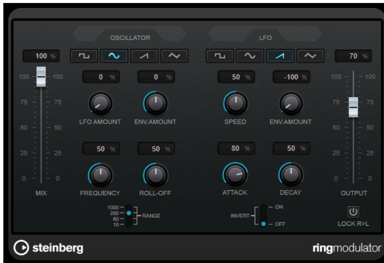
Ring modulators work by multiplying two audio signals. The ring-modulated output contains added frequencies generated by the sum of, and the difference between, the frequencies of the two signals.
