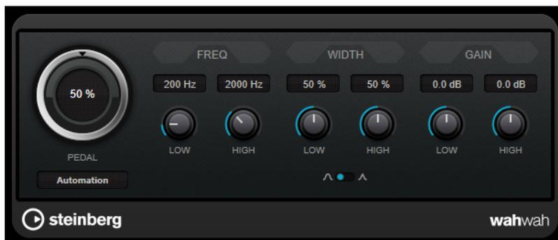
You can independently specify the frequency, width, and gain for the **Low** and **High** Pedal positions. The crossover point between the Lo and Hi Pedal positions lies at 50.
